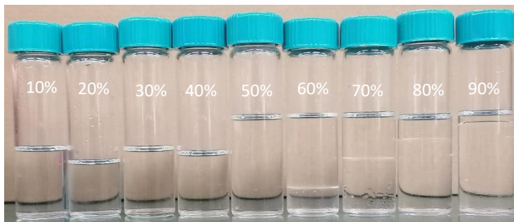
Figure 19. Eutectic-water mixtures of \text{NaC}_6:\text{C}_6(0.7) group at ambient temperature ( \sim 20^\circ\text{C} ) identified by massic content of water.
